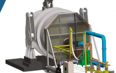
In tailor-made projects, and using the resources of our Æstus technology division, we finely adjust operational variables such as burner positioning and inclination, combustion products injection speed, path of the combustion products inside the equipment, positioning and exhaust diameter, for maximum efficiency of heating or cooling, in the various activities in which the stations are applied:
