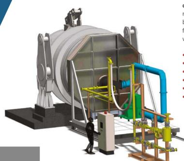
In tailor-made projects, and using the resources of our Æstus technology division, we finely adjust operational variables such as burner positioning and inclination, combustion products injection speed, path of the combustion products inside the equipment, positioning and exhaust diameter, for maximum efficiency of heating or cooling, in the various activities in which the stations are applied:
